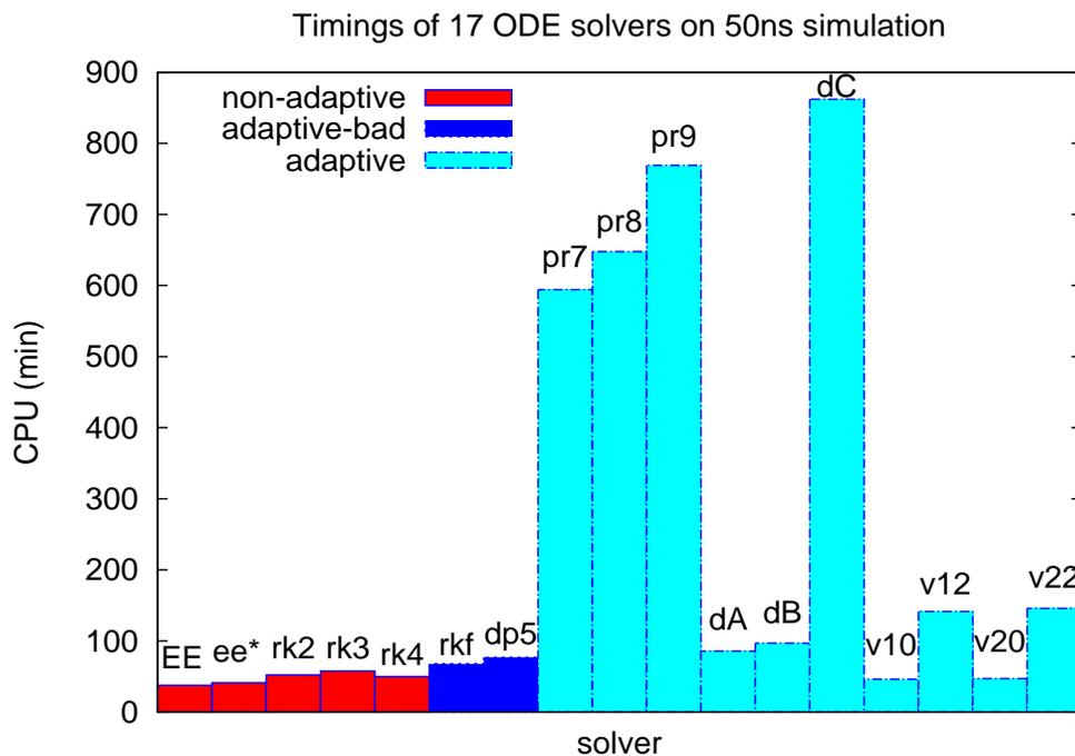
FIGURE 1. Timings of 17 ODE solvers on 50ns simulation
