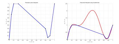
Condition of A  $\approx$  356159 Average interpolation error =  $2.7 \times 10^{-14}$ PW Linear length = 3.25 units Polynomial length = 5.38 units.
