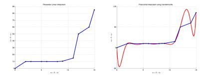
Condition of A  $\approx 1.6 \times 10^{14}$ Average interpolation error =  $1.4 \times 10^{-09}$ PW Linear length = 3.13 units Polynomial length = 559.30 units.
