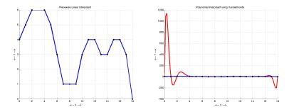
Condition of A  $\approx 1.1 \times 10^{23}$ Average interpolation error =  $7.2 \times 10^{-4}$ PW Linear length = 3.13 units Polynomial length = 559.30 units.
