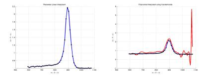
Condition of A  $\approx 2 \times 10^{146}$ Average interpolation error =  $3.6 \times 10^{-2}$ PW Linear length = 1.68 units Polynomial length = 23.47 units.
