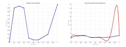
Condition of A  $\approx 4.1 \times 10^{6}$ Average interpolation error =  $2.3 \times 10^{-12}$ PW Linear length = 3.22 units Polynomial length = 37.19 units.
