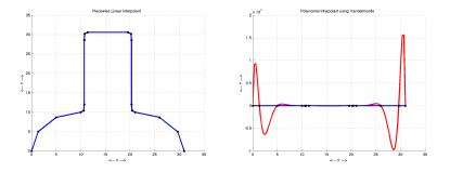
$\begin{array}{l} \mbox{Condition of A}\approx 1.3\times 10^{27}\\ \mbox{Average interpolation error}=2.9\\ \mbox{PW Linear length}=2.66 \mbox{ units}\\ \mbox{Polynomial length}=2.9\times 10^{27} \mbox{ units}. \end{array}$
